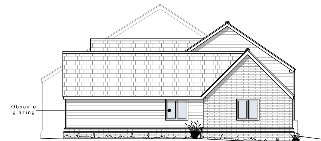
SIDE ELEVATION (SOUTH-EAST)
